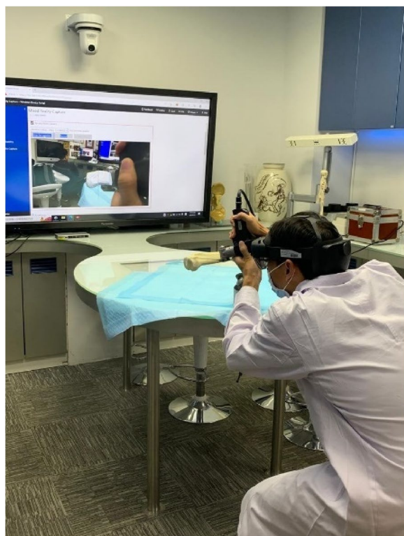
Fig. 5 Illustration of target tracking. When the tibial bone was within the visual field of Microsoft HoloLens (worn by the orthopaedic expert), target tracking was enabled to achieve the overlaying
