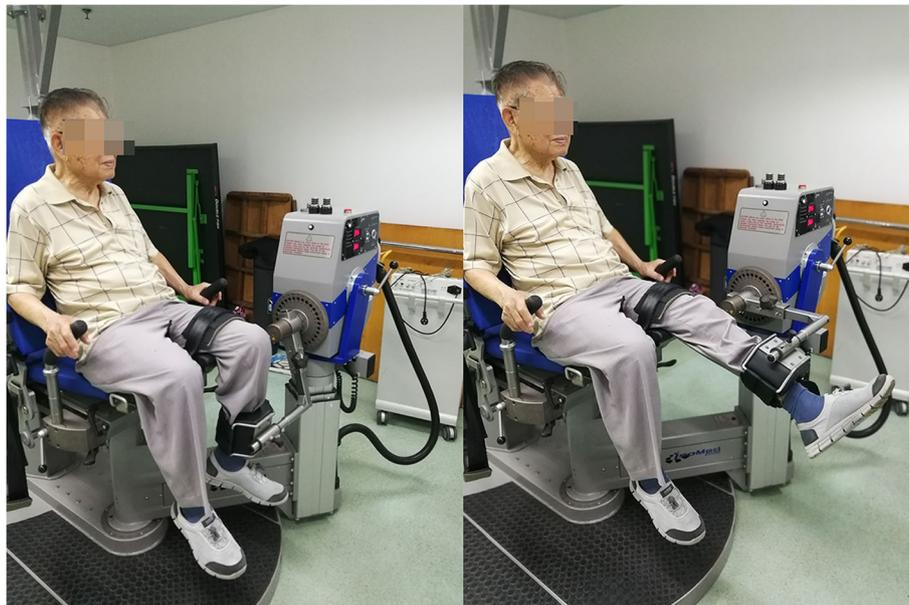
**Fig. 1** Isokinetic torque measurement with the IsoMed 2000 dynamometer
