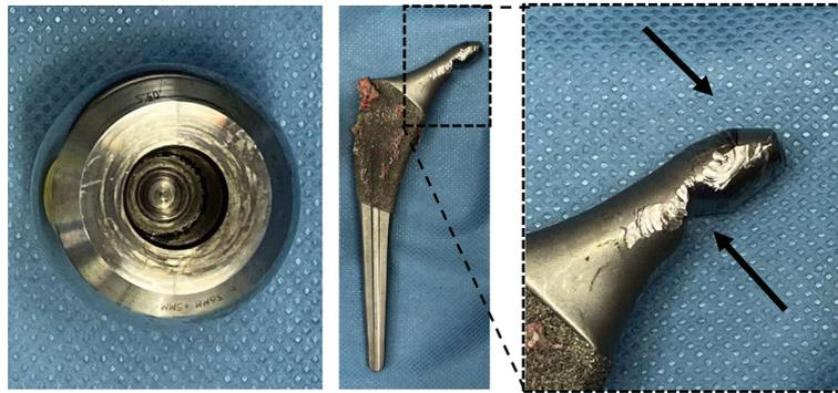
**Fig. 4** Photographs of the extracted instrumentation. Left panel: metal debris inside the metal head. Middle and right panels: significant deformation at the head-stem trunnion (arrows)
